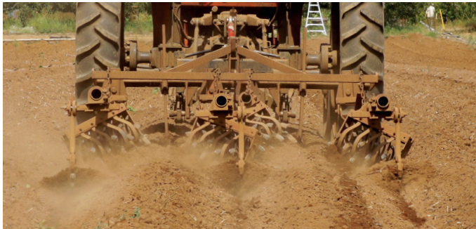
FIGURE 1. Rolling cultivator. Photo: Jim Clark
